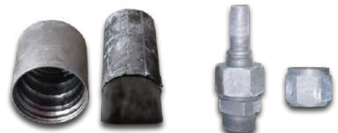
E-Coat 1000 after 1,000 hours ASTM B117 (ISO 9227) salt spray test
