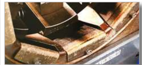
Sliding bearing in condition after ca. 900.000 crimping operations
